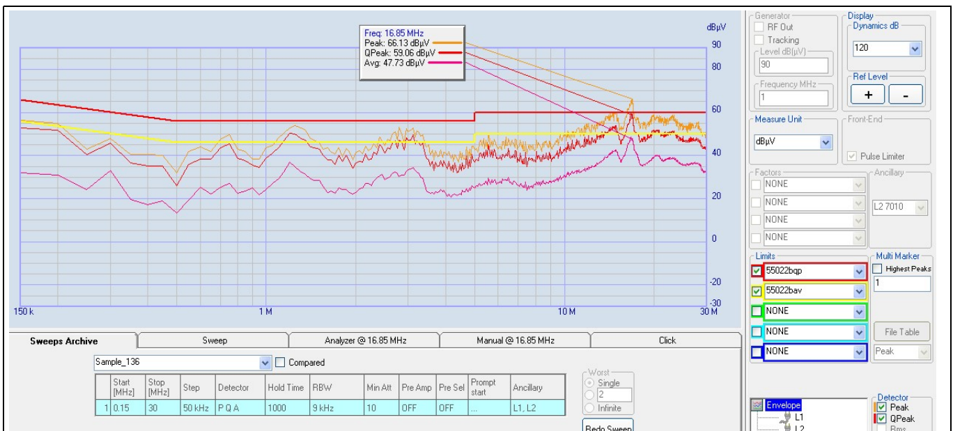
Figure 53 Conducted emissions at 230 V AC RMS with 100 percent load
